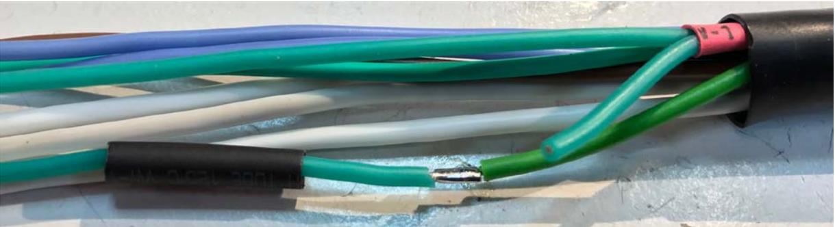
Solder the two wires as in the picture above
